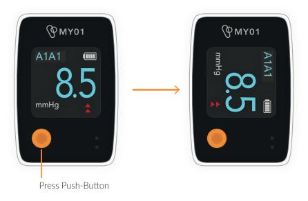
Figure 5: Rotating Display Orientation
