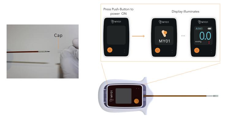
Figure 12: Removing Needle Cap and Turning ON the Pressure Monitor
