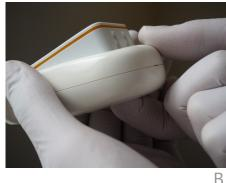
Figure 15: Ejecting the Pressure Monitor
