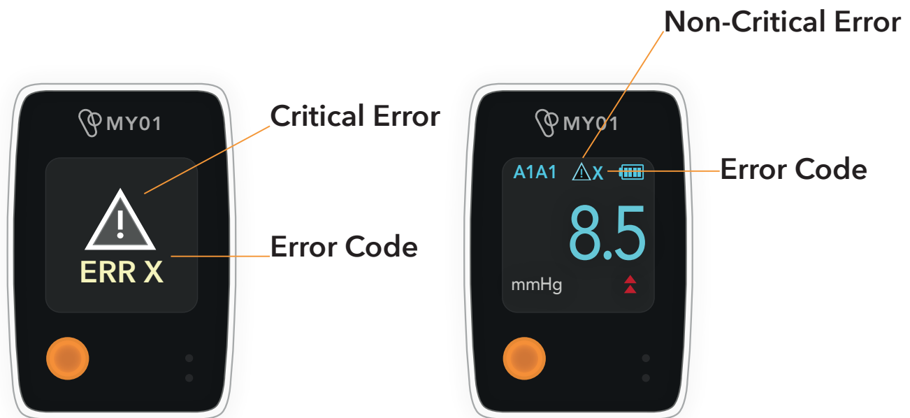
Figure 13: Error Code Display
