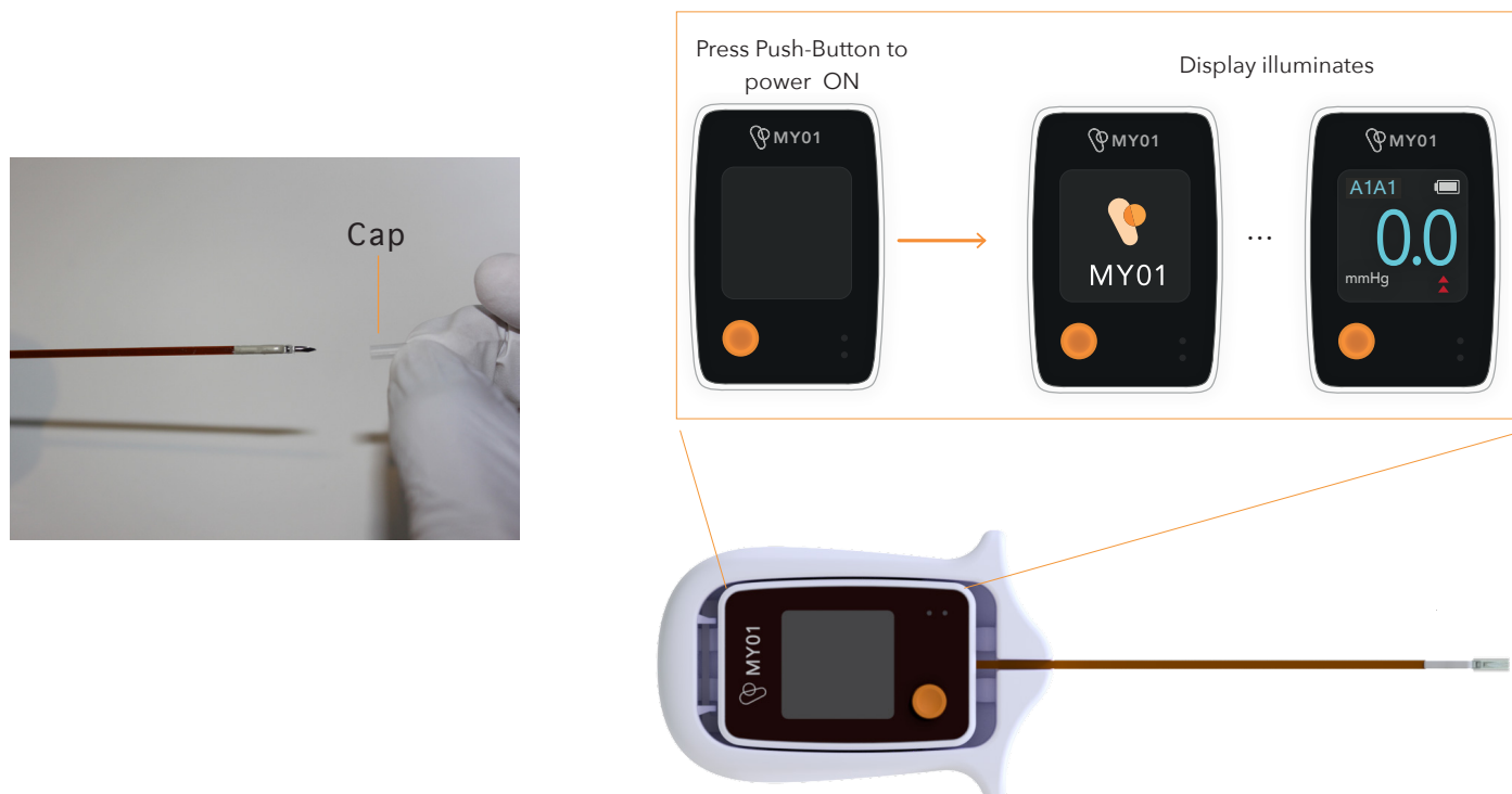
Figure 6: Removing Needle Cap and Turning ON the Pressure Monitor
