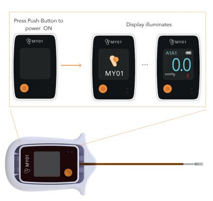
Figure 6: Removing Needle Cap and Turning ON the Pressure Monitor
