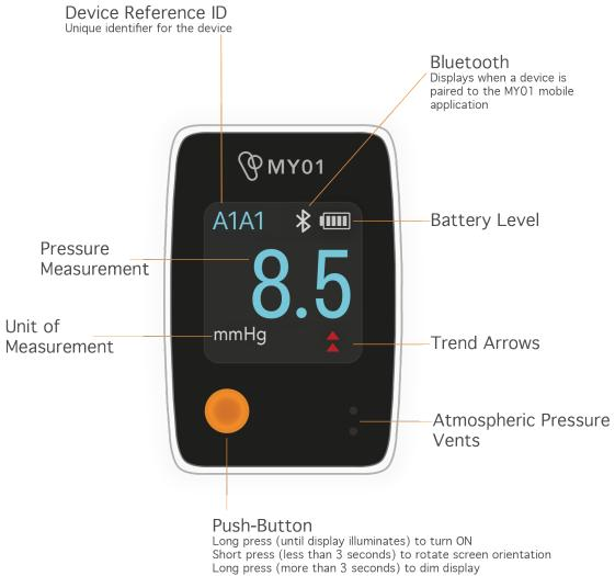
Figure 4: Device Controls and Display Icons
