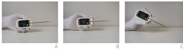
Figure 7: Recommended Device Grips
